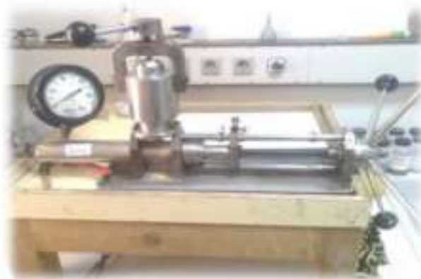
Figure (13) : Pompe volum trique   mercure (CRD 2018).
