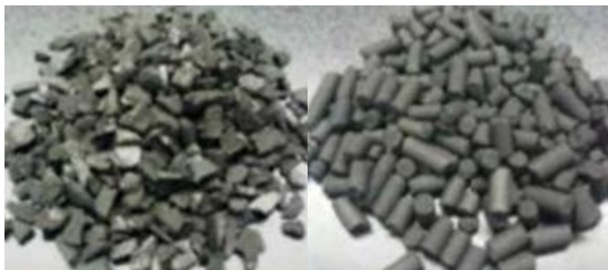
Figure II.3 : Granular Activated Carbon
