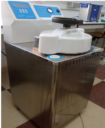
Autoclave (raypa steam sterilizer).
