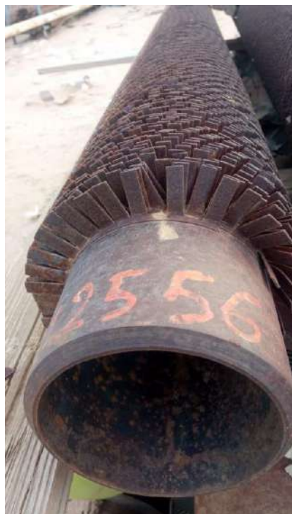
Figure 07: tubes de zone convection et radiation de four BA-201
