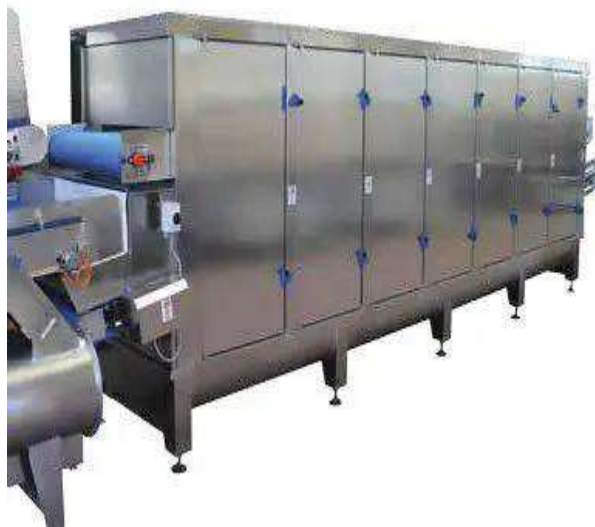
Figure I. 3 Tunnel de séchage [48]
