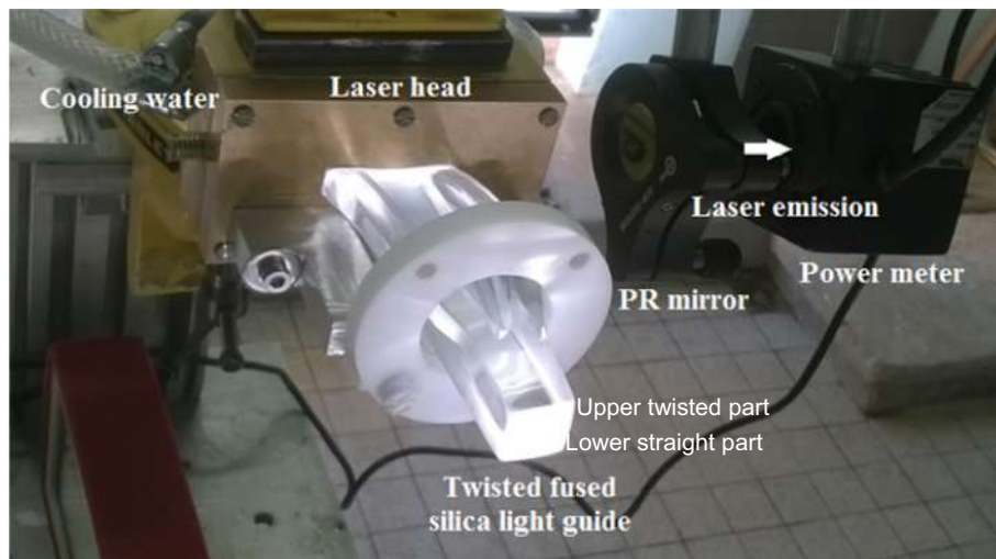
Fig. 2. Solar-pumped Nd:YAG laser head composed of the monolithic light guide, the solar laser head and the laser resonant cavity.
