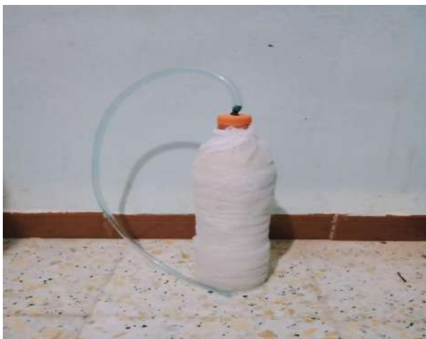
Photo N° IV.15: Bottle wrapped in a geotextile fabric
