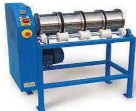
Figure III .8. Machine micro deval [28]
