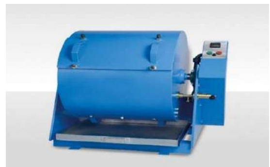
Figure III .7. Machine los Angeles [27]
