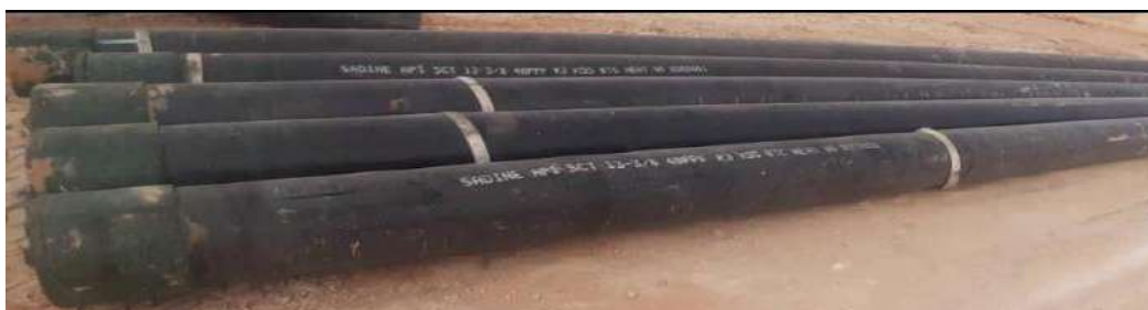
Figure II.10 : tubage en acier 133/8'
