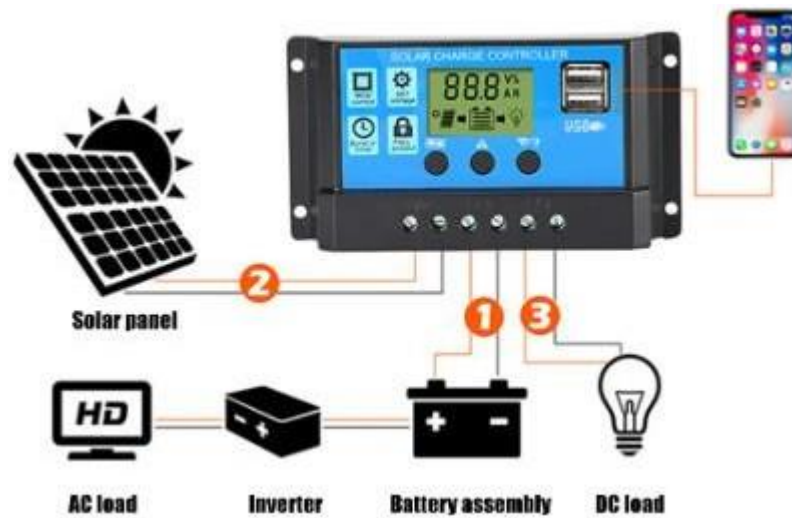
Figure.I.12 Components and connections of the photovoltaic system [15].
