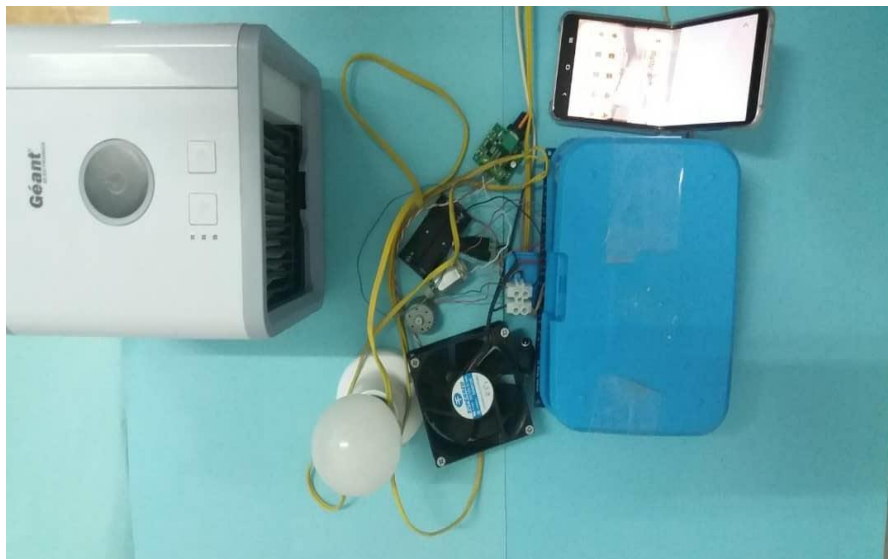
Figure.III.28: The realized device to control real appliances of smart home
