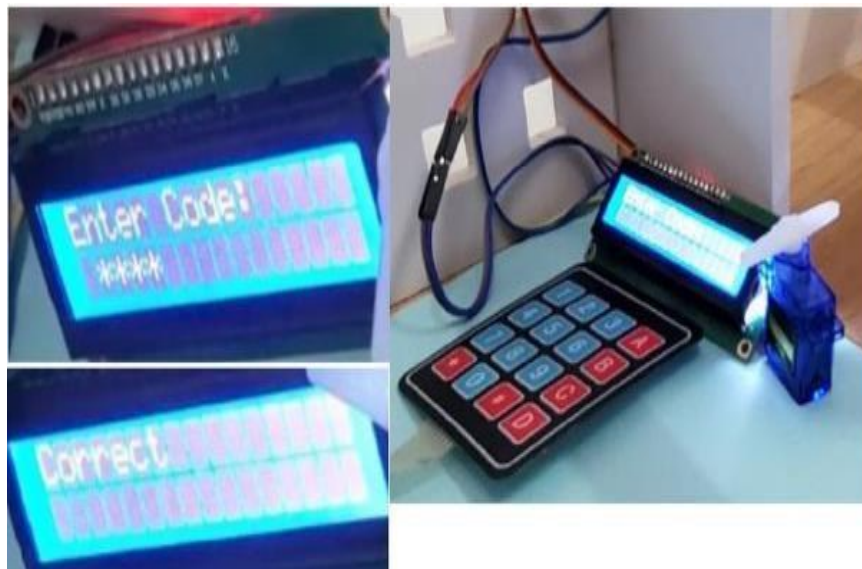
Figure.III.1: Implementation and testing of the door lock system
