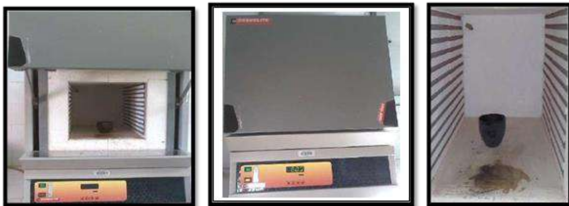
Figure 53 : Muffle oven with platinum crucible (Matrix acidizing technique, laboratory testing- Sonatrach, 2020).
