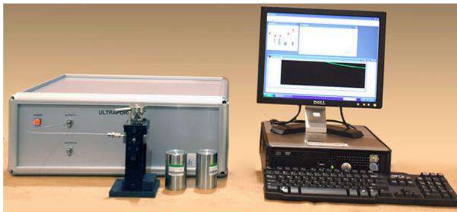
Figure 43 : UltraPore Porosimeter - UPore 300 (Matrix acidizing stimulation technique, laboratory testing Sonatrach, 2020).
