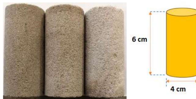
Figure 37 : Some sandstone plugs from well N1 and its dimensions (Sonatrach/ EP HBK, 2020).
