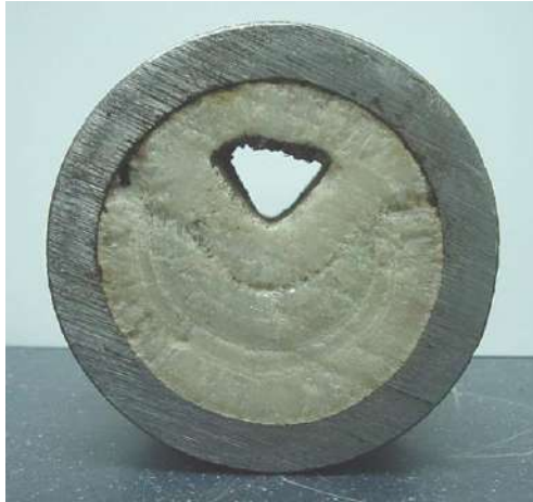
Figure 13 : An example of deposited calcite (Sonatrach/ EP HBK, 2020).
