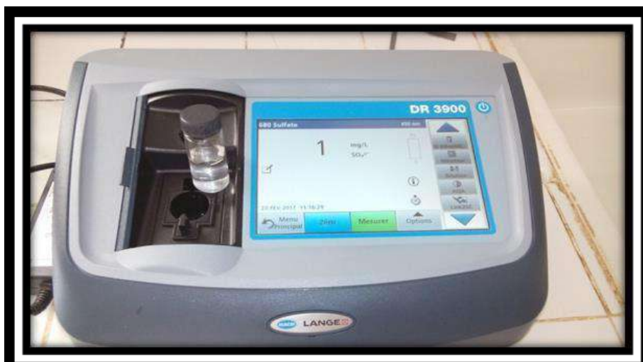
Figure 59 : DR 3900 spectrophotometer with sulphate cell (Matrix acidizing technique, laboratory testing-Sonatrach, 2020).
