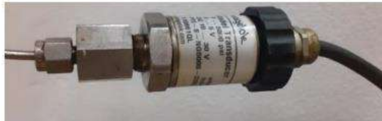
Figure 50 : Pressure transducers (Matrix acidizing stimulation technique, laboratory testing Sonatrach, 2020).
