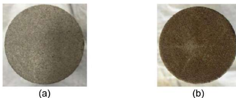
Figure 15 : Sandstone core face after acidizing (a) without iron (permeability improved) and (b) with iron (permeability damaged) (Rady and Nasr-El-Din, 2015).
