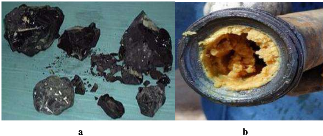
Figure 16 : a. Some Asphaltene samples b. Deposited Praffins (Sonatrach/ EP HBK, 2020).
