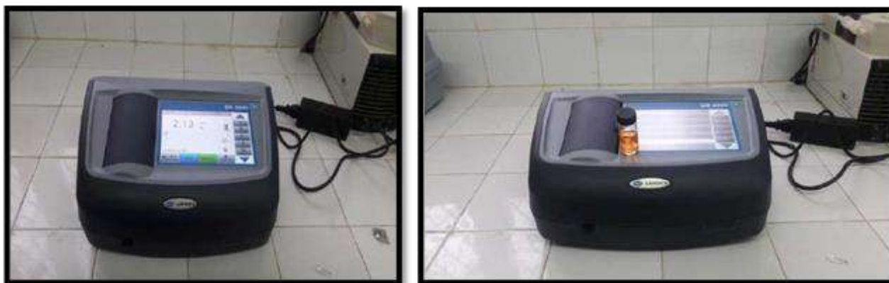
Figure 58 : DR 3900 spectrophotometer with iron cell (Matrix acidizing technique, laboratory testing-Sonatrach, 2020).
