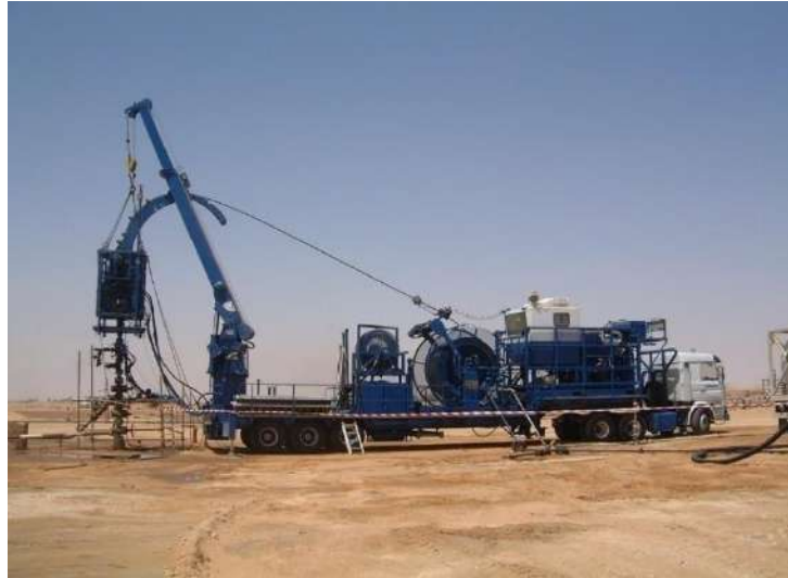
Figure 30 : Coiled Tubing unit of Schlumberger Company.
