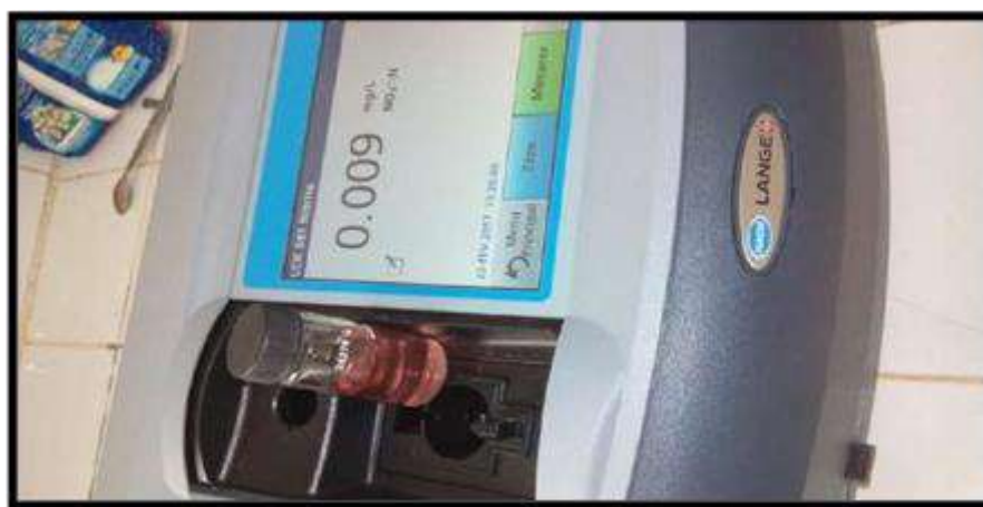
Figure 60 : DR 3900 spectrophotometer with nitrite cell (Matrix acidizing technique, laboratory testing-Sonatrach, 2020).
