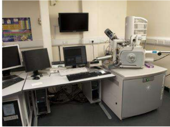
Figure 42 : Microscope Electronique à Balayage (Quanta 650) (Matrix acidizing stimulation technique, laboratory testing Sonatrach, 2020).
