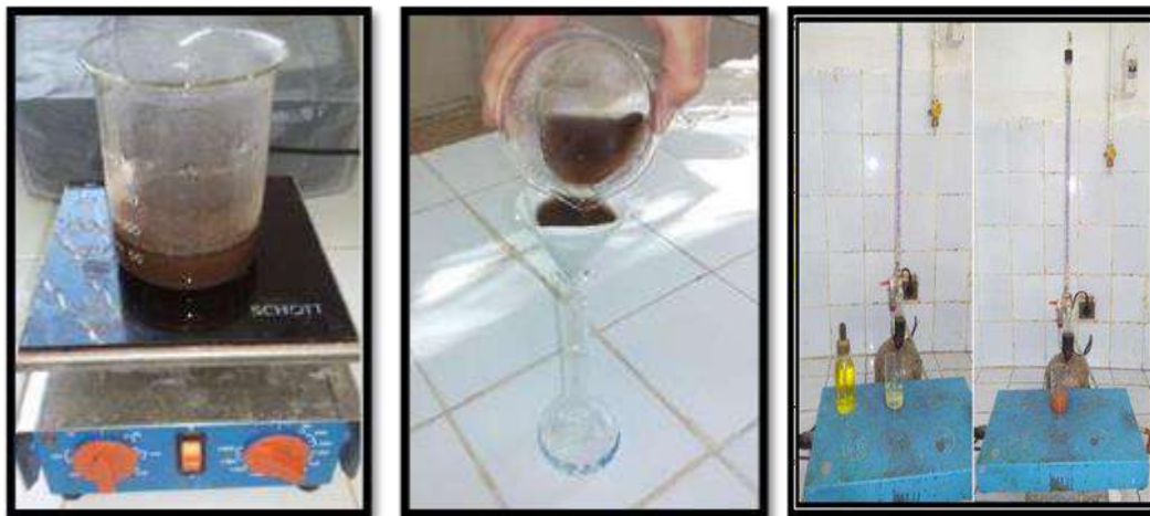
Figure 54 : A conical flask with filter and a burette (Matrix acidizing technique, laboratory testing- Sonatrach, 2020).
