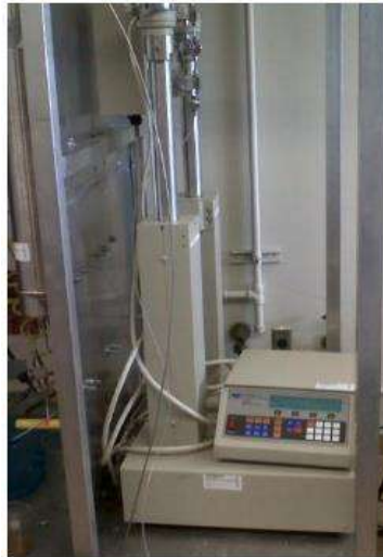
Figure 47 : Syringe pump Continuous Flow 260D Teledyn ISCO Dual Syringe Pump and controller (Grabski, 2012).
