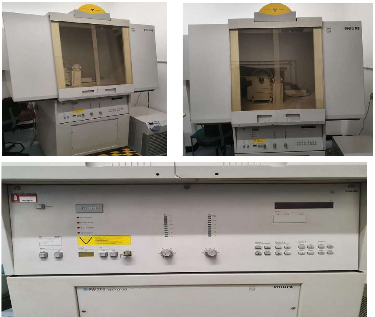
Figure 40 : XRD equipment (Matrix acidizing stimulation technique, laboratory testing Sonatrach, 2020).
