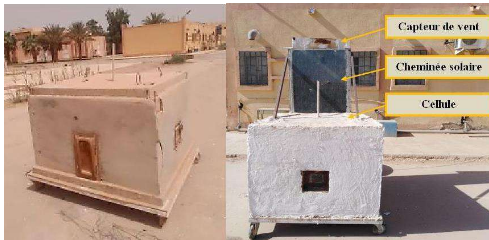
Figure II. 1: Descriptions de la cellule.
