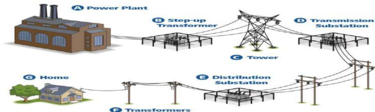
Figure I.3: Organization of the power system[11]
