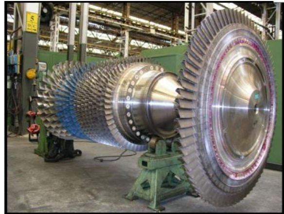
Figure 2.9: Axial compressor section and The HP wheel
