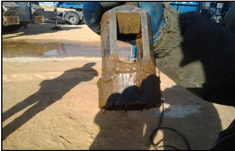
FigureIV- 14: Gauge cutter (GC86 mm).
