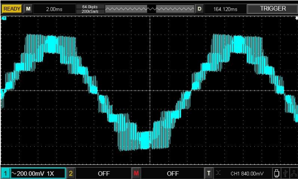
Fig III.21: Experimental results of the output voltage of the 5-level DCC using different PWM techniques, (a): PD, (b): POD, (c): APOD and (d): SSVM
