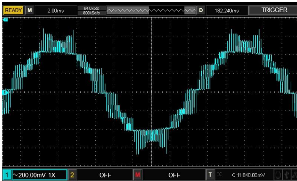
Fig III.22: Experimental results of the output voltage of the 7-level DCC using different PWM techniques, (a): PD, (b): POD, (c): APOD and (d): SSVM
