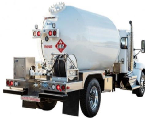
Figure 18: Camion-citerne de propanes.
