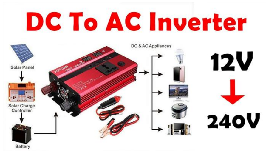
Figure 1.7 An illustrative explanation of the role of an inverter in a renewable energy system.
