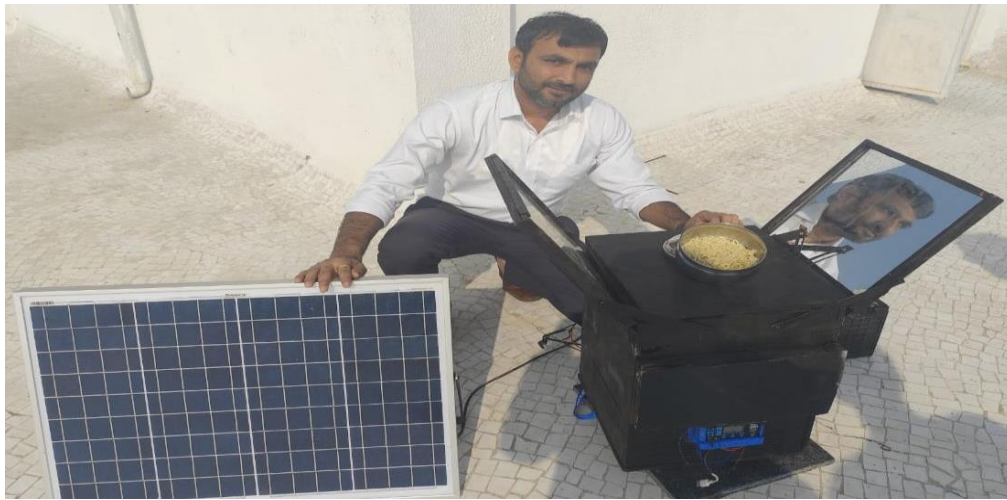
Fig II.3: Experimental setup with arrangements and battery [36].
