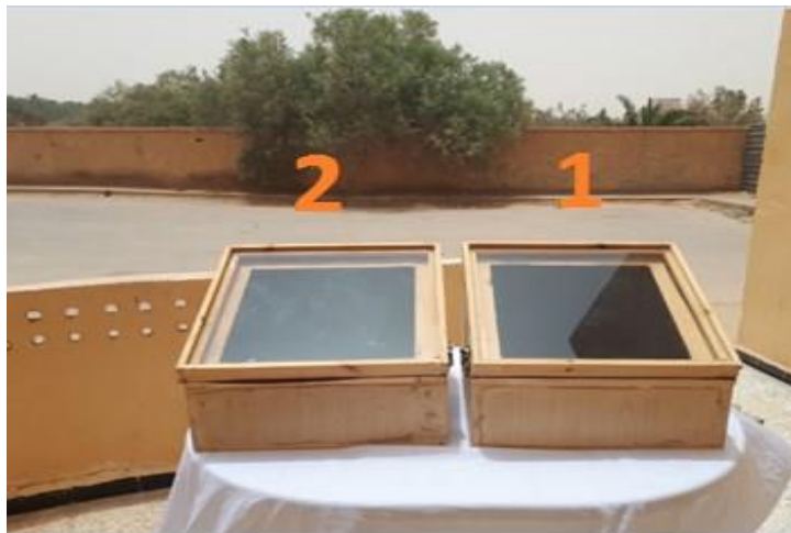
Fig II.1: Experimental Solar Box Cookers Used for Determining Optimal Volumetric Efficiencies (VE1 and VE2) [34].
