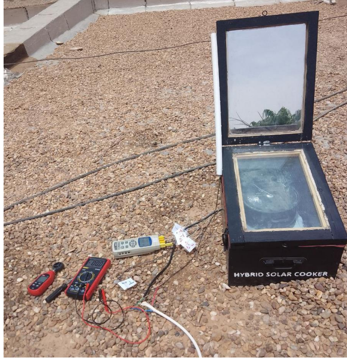
Fig III.11: Real picture of the hybrid solar cooking system.
