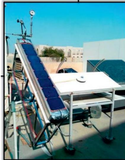
Figure II.13 Cooling system with convergent heat exchanger[66].
