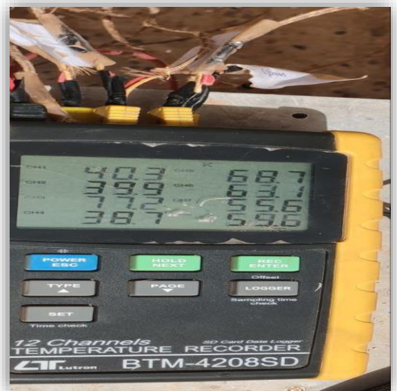
Figure II.27 : Photograph of the 12-channel temperature recorder
