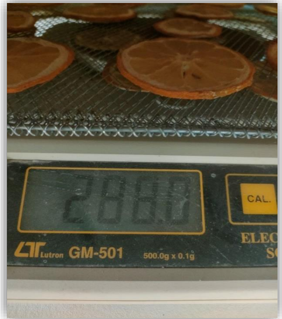
Figure II.26: Lutron gm-500 digital scale, 500g x 0.1g, rs-232
