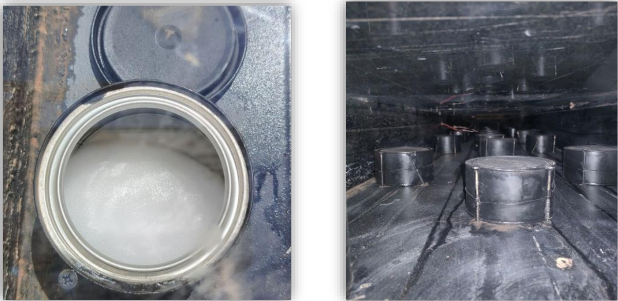
Figure II.21 : The paraffin that was used in the thermal energy storage system
