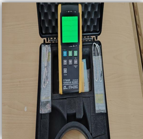
Figure II.27 : Photograph of the 12-channel temperature recorder
