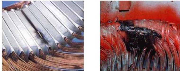
Figure 1.8: Examples of damage brought on by short circuits in IM stators
