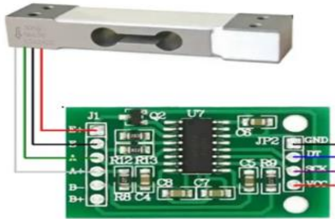
Figure.3.1: Electrical wiring between the load cells and the Hx711 module
