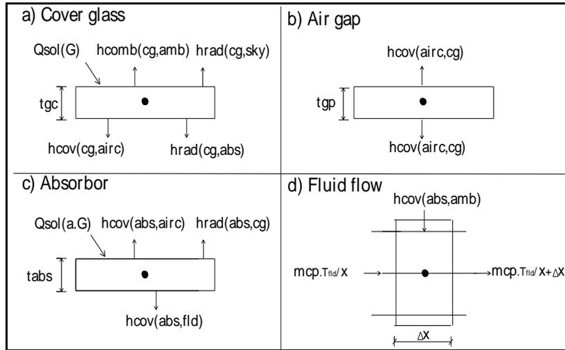
**Figure I.2b: Single glazed flat plate solar panel heat mechanism.**
