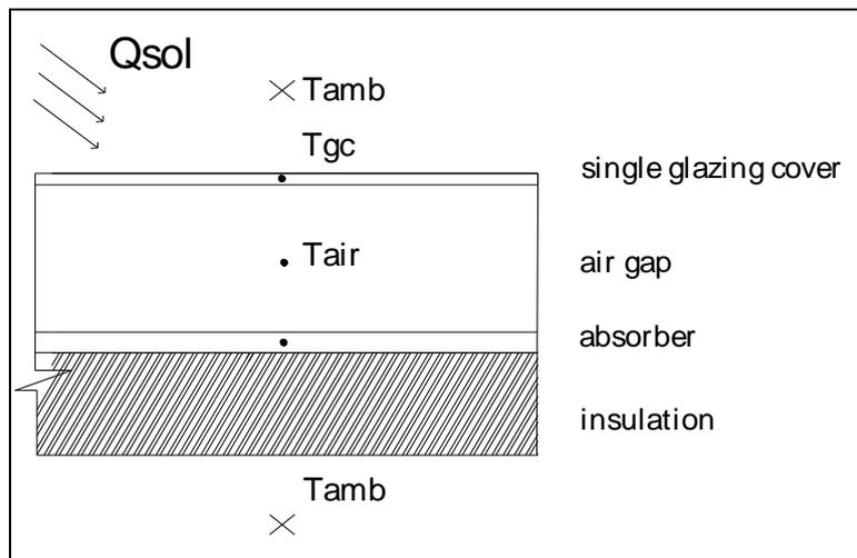
**Figure I.2a: Single glazed flat plate solar panel temperature distribution.**
