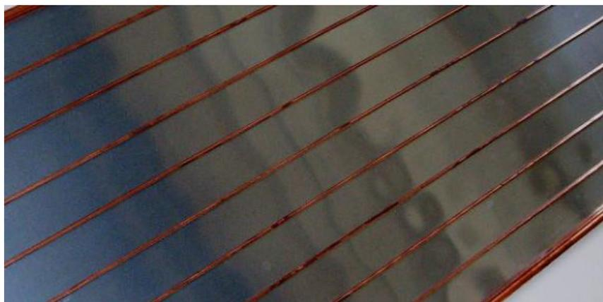
**Figure I.2: Laser welding absorber.**
