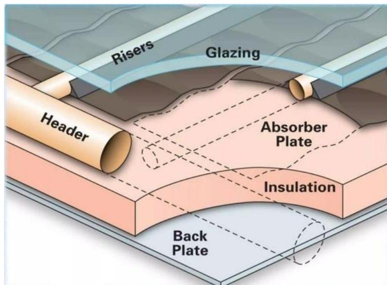
**Figure I.1b: Components of solar flat plate collector**
