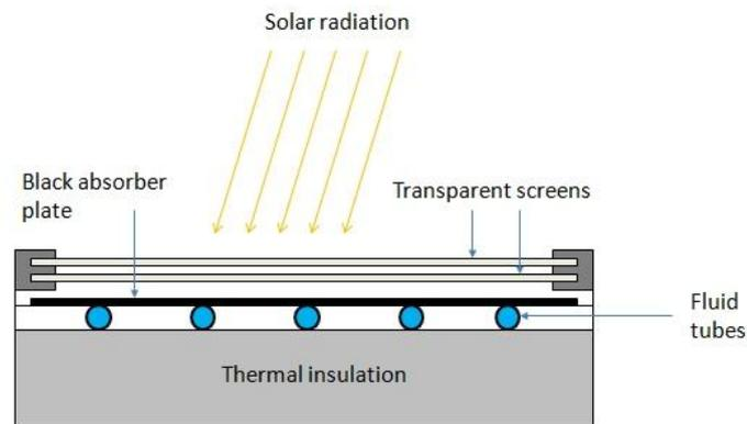
**Figure I.1a: Schematic of a plate solar collector with transparent screens**
