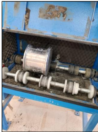
Photo II. 2 : La machine micro-Derval.
