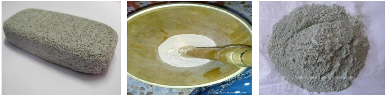
Figure II-7: Preparation of pumice powder
