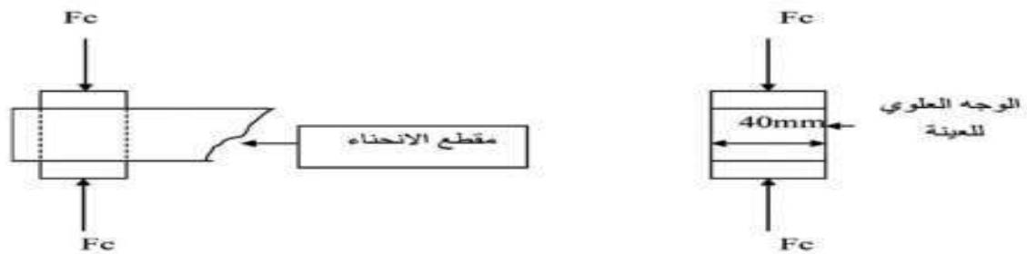
Shape III-9: Illustration of the pressure crushing mechanism
