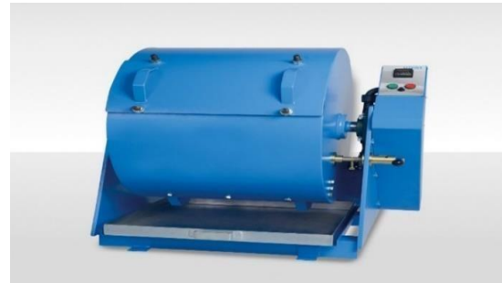
Figure 3.5. Machine los Angeles
