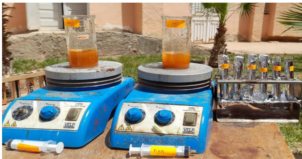
Figure(III-10): Photo of a photocatalysis study of CuO-sand ,MgO-sand catalyst
