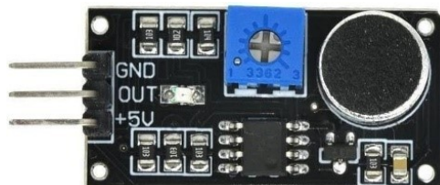
Figure 2.3: Sound Sensor module LM393
