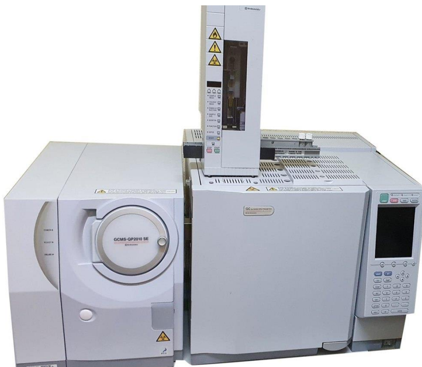
FIGURE III.1. SHIMADZU GCMS-QP2010 SE INSTRUMENT USED FOR FATTY ACID ANALYSIS
