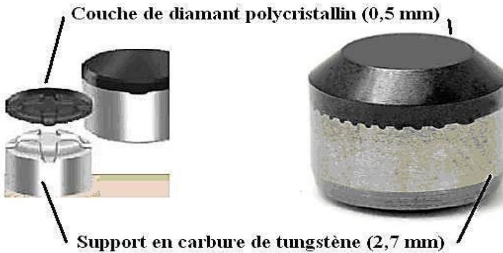
Figure I.16: Structure d'un PDC
