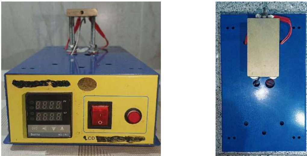
Figure 2.2: The homemade spray pyrolysis technique (SPT) system.
