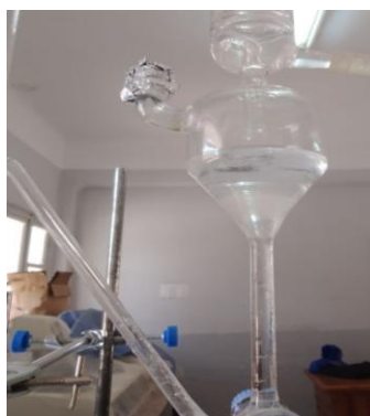
Figure (III-2): Hydro-distillation setup showing the accumulation of the essential oil.
