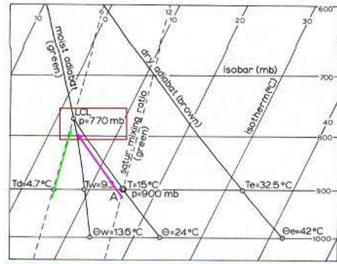
Figure (II.7): Illustration of the Lifted Condensation Level (LCL) on a Skew-T Diagram [18].
