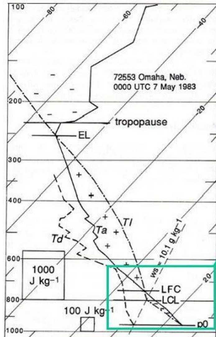
Figure (II.8): Determination of the Level of Free Convection (LFC) on a Skew-T Diagram [18].
