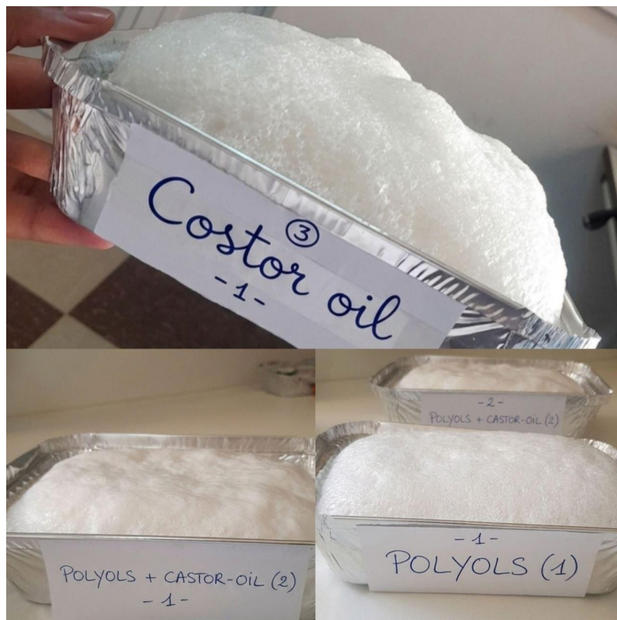
Figure III.5: Expanded polyurethane foams in aluminum molds
