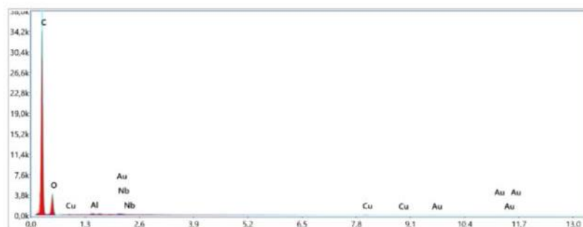
Figure III.8: EDX spectrum of coffee grounds
