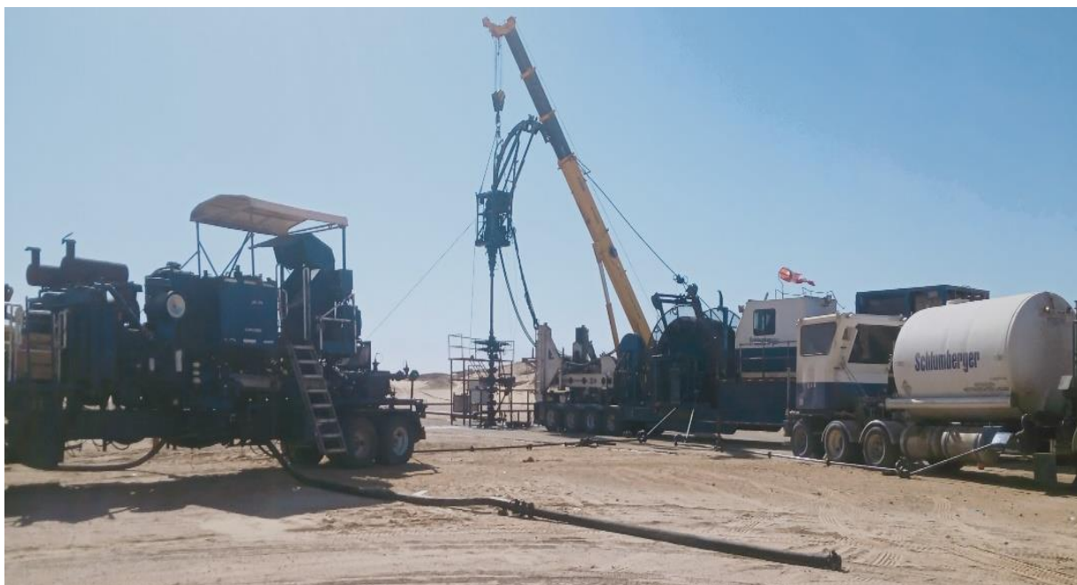
Figure III.8: Coiled Tubing Site (Equipment spotting).
