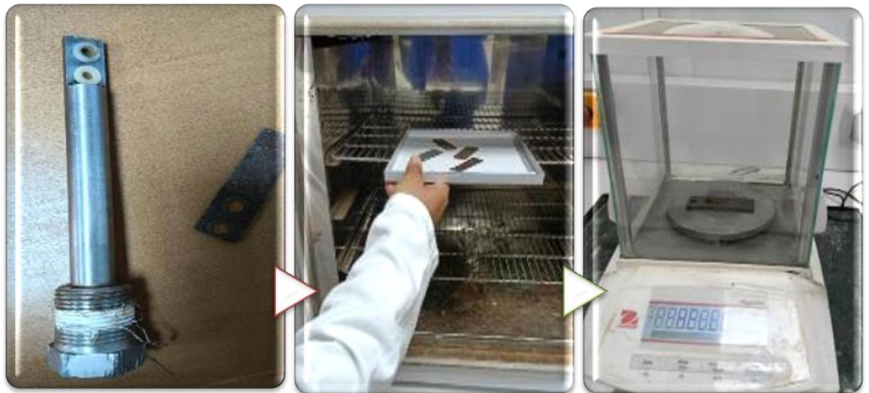
Figure III.3: Traitement des coupons
