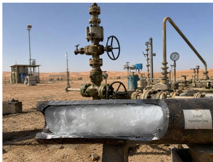
Figure III.4: AI-generated illustrative image showing hydrate blockage inside a gas lift injection line.
