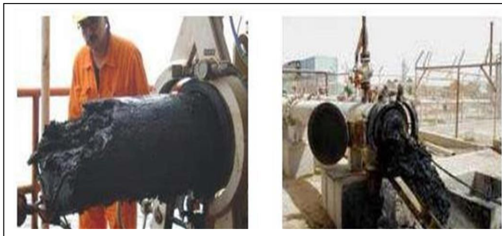
Figure I. 7 Asphaltene deposit in the production tube (2)
