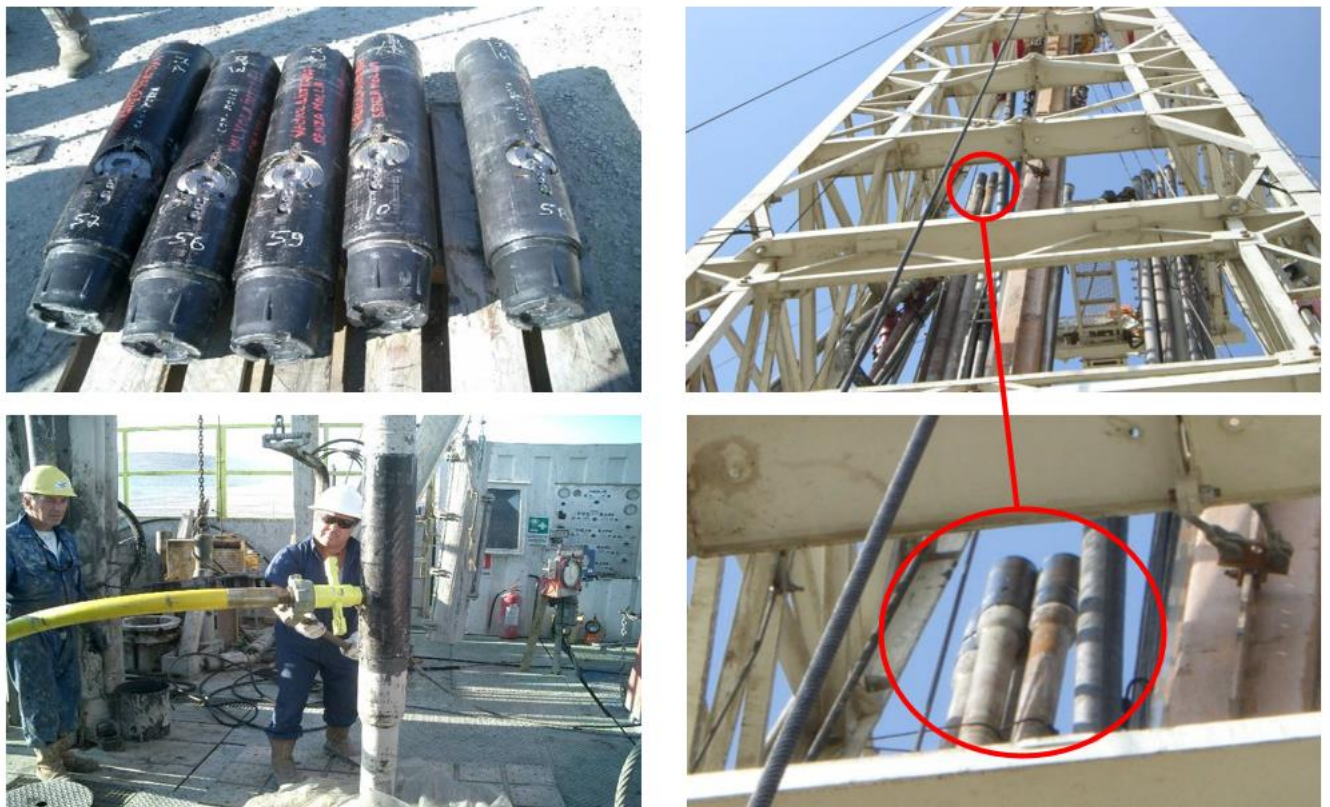
Fig.II. 2: The E-CD Sub: Surface Handling, Rig Integration, and Stand Installation [3].
