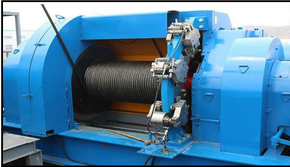
Figure.20. Le treuil (ou drawworks)
