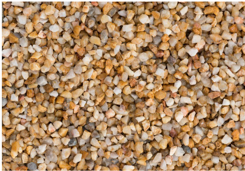
Figure .32 Massif filtrant
