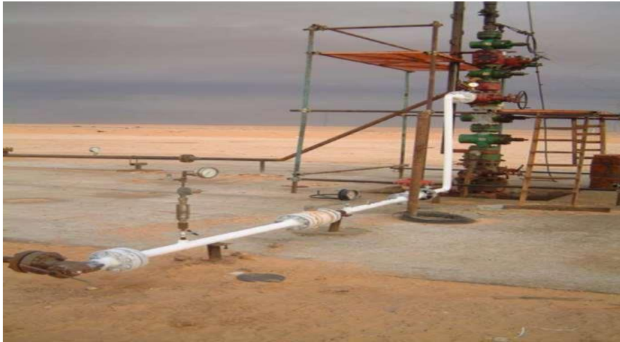
Figure 9: Complétion Gas-lift direct
