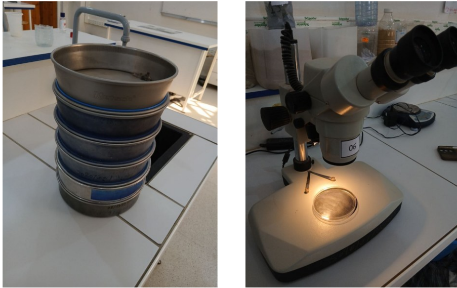
Figure 4 : Principal equipment used for sediment treatment and observation
