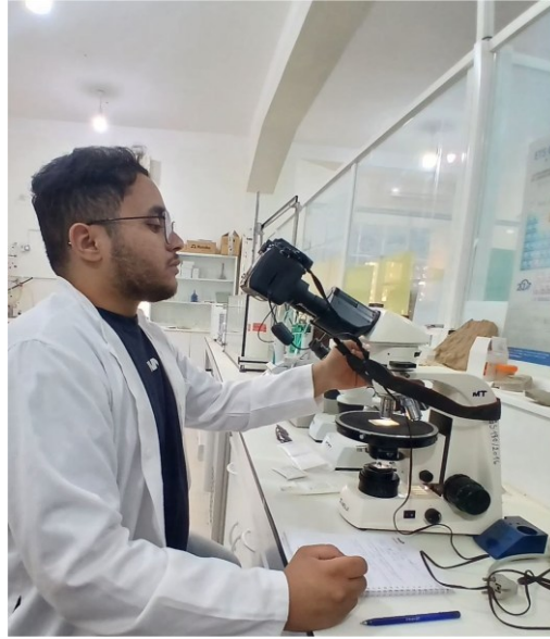
Figure 5 : Petrographic observation and analysis of thin sections utilizing specialized laboratory equipment at the research center(Kasdi Merbah university).
