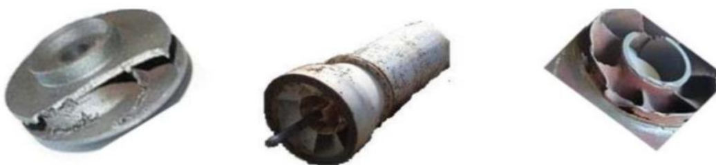
Figure 0-14 : Cavitation damage to the components of a centrifugal pump
