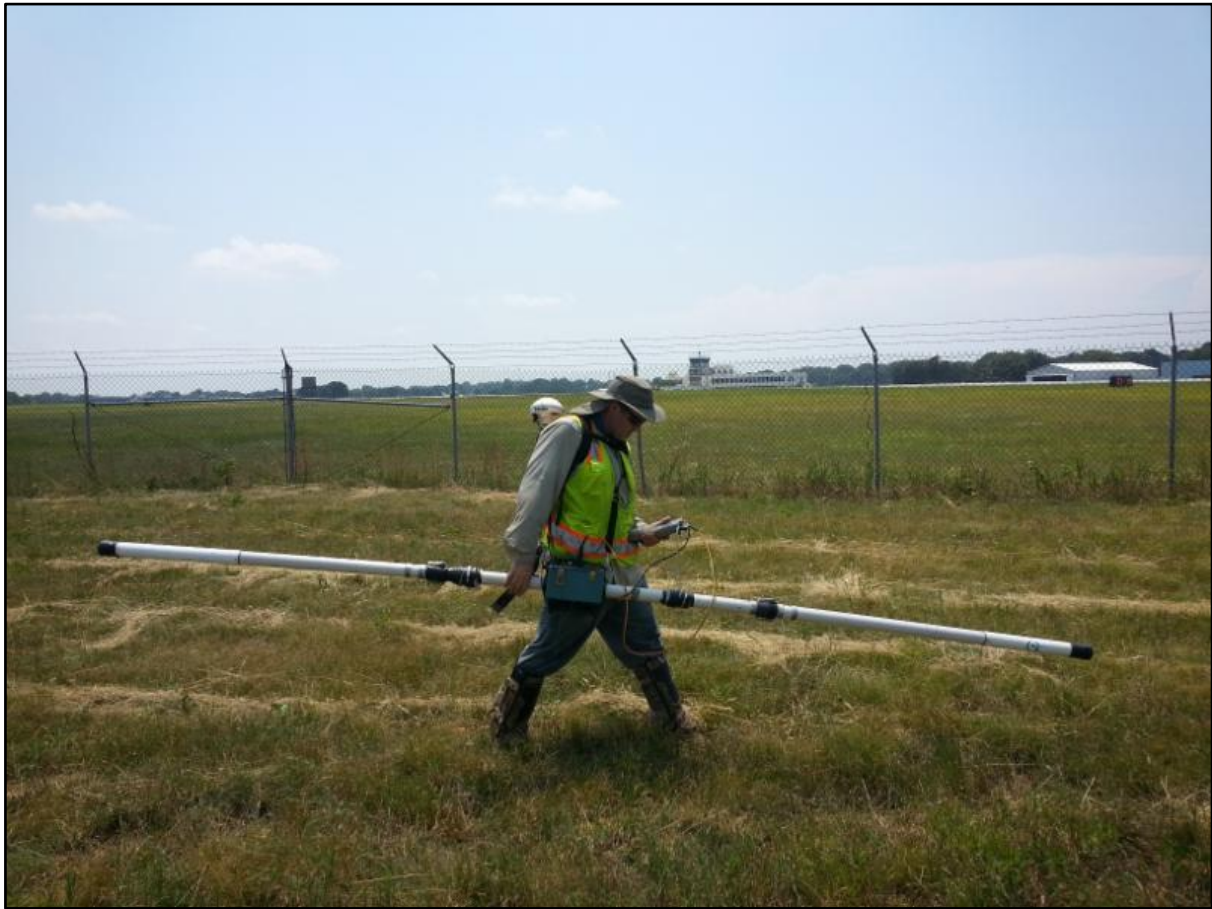
Figure 5: Geonics EM31 Ground Conductivity Meter. The instrument showing transmitter and receiver coils at fixed separation (Source: Pyramid Environmental ).
