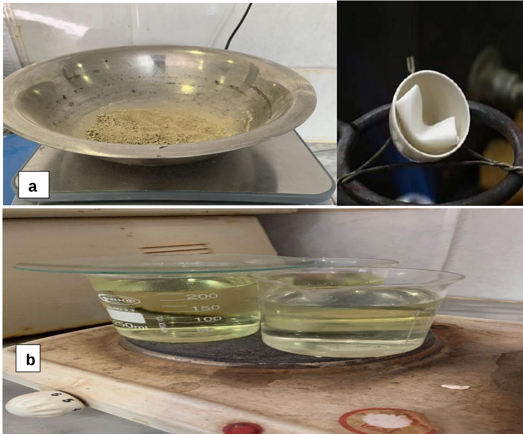
Figure 9: Shows a) Drying, pulverizing, and sieving of aggregate sample, b) Boiling with HCl, cooling, and filtration of solution, c) Precipitation of \text{BaSO}_4 and calcination in crucible.
