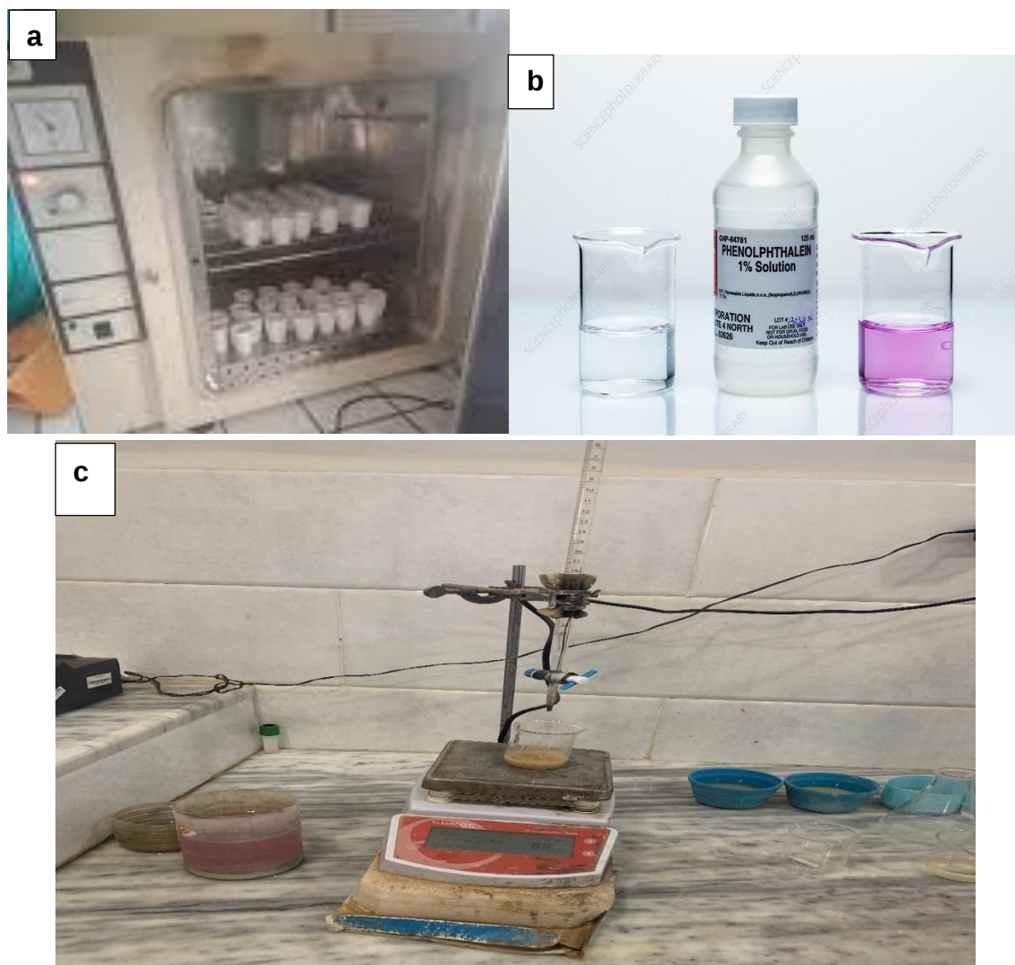
Figure 8: Shows a) Oven-drying of aggregate sample at 105–110 °C, b), c) Titration with \text{NaOH} solution showing color change.
