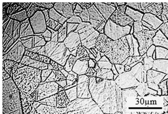
Figure I.4 :AISI 316L austenitic stainless steel microstructure
