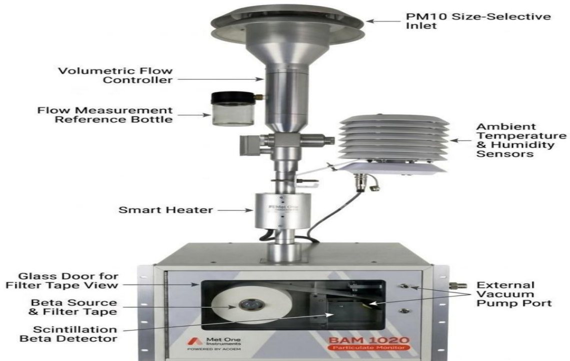
Figure 3.3 – Detailed component layout and assembly of the Met One BAM-1020 particulate monitor. [32].
