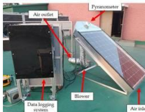
Figure II.4: Bench setup of the PV/T air-cooled system showing the integration of data acquisition and solar monitoring instruments
